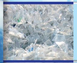
The labels and caps are removed, then the bottles are washed, crushed and chopped into small pieces called "flake".
